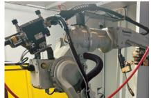
In addition, Dura Manufacturing boasts a full robot welding facility with twin Panasonic robots and two automated jigs. This tandem robot welding system brings speed, consistency and quality. Parts are precisely aligned on a jig before the dual welding arms use their optical sensors to follow a pre-programmed path to delivery consistent, high-quality welds on materials of varying thicknesses. This system allows for simultaneous loading and unloading, meaning production flows continuously.
