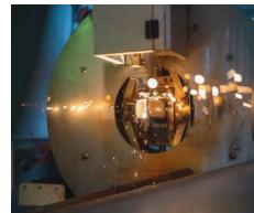
Dura Manufacturing's 9kW Amada Regius laser can pierce a **25mm steel surface in 1 second** and has an X/Y positioning speed of 340m/min
